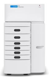
The unique design features of the Fragment Analyzer instruments combines ease of use automated electrophoresis with the flexibility to switch between DNA and RNA analysis kits without maintenance between runs. The reagent kit portfolio covers a broad range of applications and offers efficient solutions for separating and analyzing nucleic acids.
