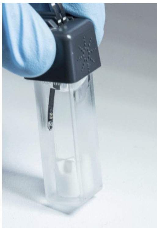
Figure 2. The in-cuvette temperature probe, used to control experimental temperature during the measurements.
