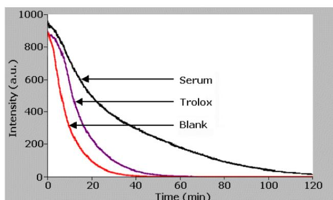
Figure 2. Fluorescence intensity vs. time for the free-radical attack of R-PE by AAPH (1) with protection by antioxidants (from human serum) or trolox and (2) without antioxidant protection (Blank)
