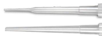
Comparison between a standard 250 µL tip with 0.61 mm (0.024 in) opening (upper) and a wide bore tip with a 1.52 mm (0.060 in) opening (lower).
